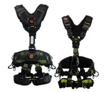
Flyer Pro PES Webbing 45mm water repellent Aluminum alloy D-ring at: front/back/ventral/sides Comfort padding - Lite - Air - Reflective Seat connection points 4 aluminum Izy buckle, 5 steel bar buckles, 9 adjustment points, 5 tool holder points Lanyard parking attachment. Fall Indicator - Legs Series #FS243.2IP
